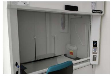
below 100 fpm, a warning label will be posted on the sash of the fume hood and Physical Plant will be notified to correct the problem.
